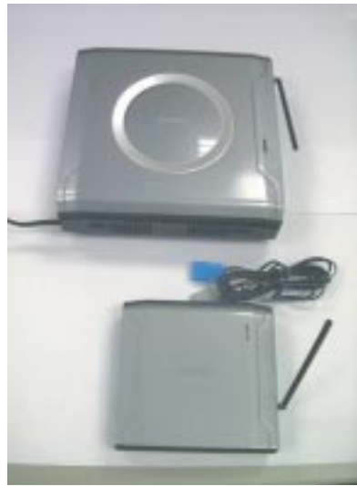
Figure 1-1 Wireless transm. receiver cabinets
